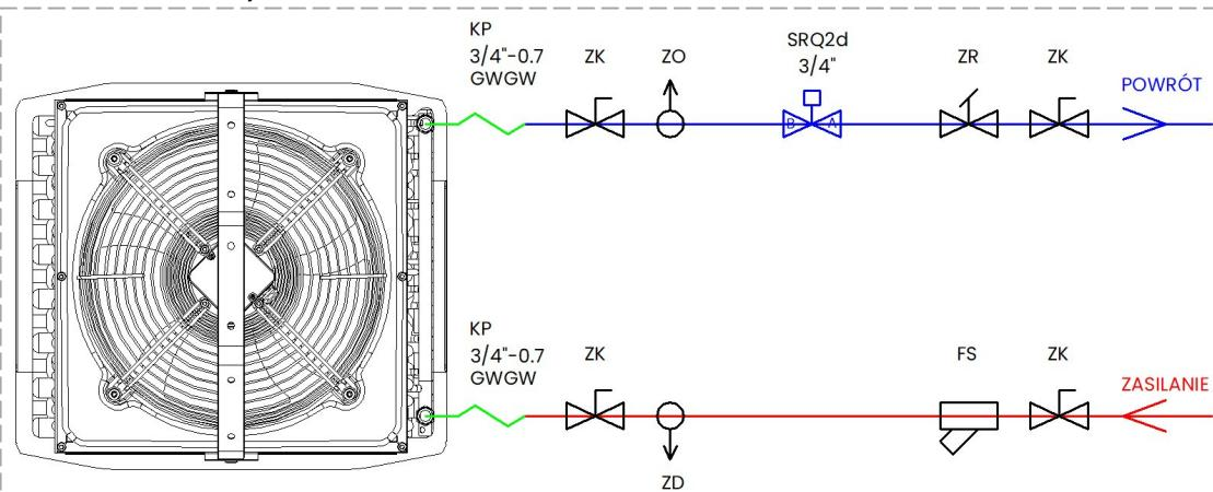
**ZK**-shut-off valve; **ZO**-vent valve; **ZD**-drain valve; **FS**-mesh filter; **ZR**-balancing valve;
