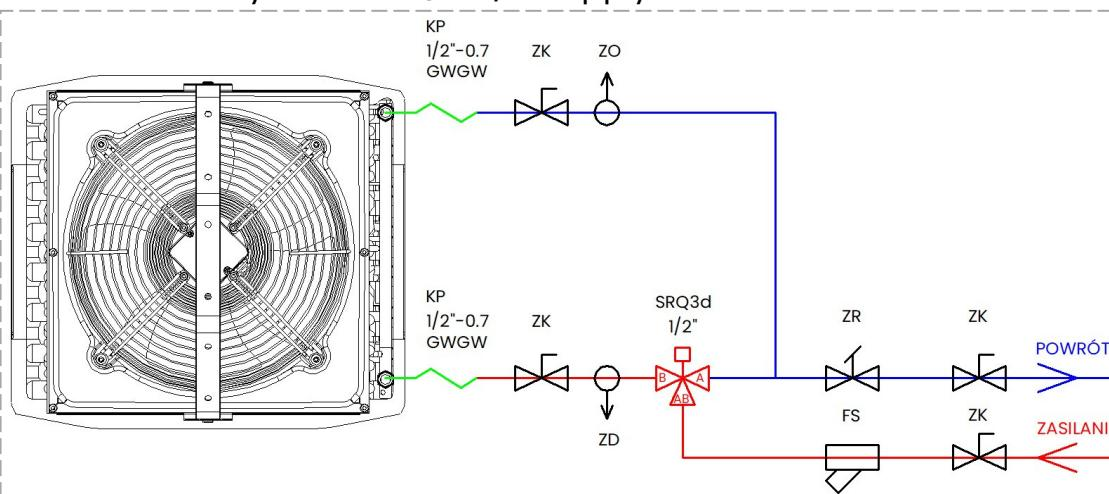
**ZK**-shut-off valve; **ZO**-vent valve; **ZD**-drain valve; **FS**-mesh filter; **ZR**-balancing valve;
