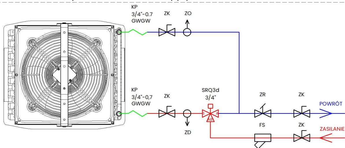
ZK—shut-off valve; ZO—vent valve; ZD—drain valve; FS—mesh filter; ZR—balancing valve;
