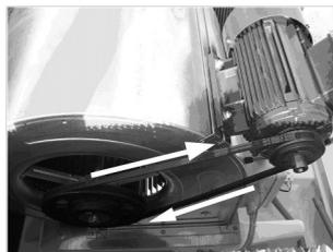
4. If the fan should rotate in the wrong direction, it's necessary change the main switch power supply connections by exchanging L1 and L2 connections
