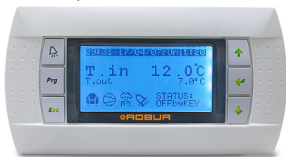
Figure 1.3 PGD control panel
