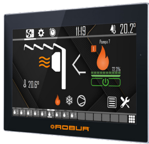
Figure 1.5 Multi RCC control panel
